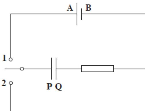
The switch is moved to position 1 until the capacitor is fully charged. The switch is then moved to position 2.
